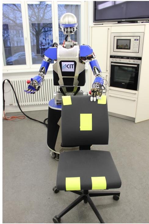
Figure 2.5: ARMAR III grasps chair using visual servoing. Yellow spots are markers which are used in early implementations, but will be removed in a later stage as soon as more advanced visual recognition and localization approaches are ready for integration in the final demonstration
