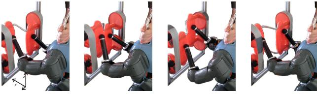
Fig. 5. Image sequence showing approximately one period of rotating the vertically mounted pedal racer with the arms of the COMAN robot after the learning, when the contact with the pedals is constantly kept. The attached video shows the complete experiment. The tape on the wheels simulates contact with the ground and keeps them at the same velocity, preventing the device from locking up, which happens if the front and the back wheels do not rotate together.
