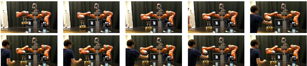
Figure 3.4: Sequence of images showing modification of robot motion though force-based exploration and on-line modification of robotic motion using force feedback while the robot is maintaining the contact with the table.
