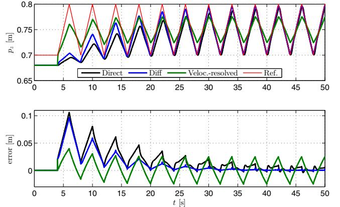
Fig. 4. The results of simulated trajectory adaptation using three different control methods, with a tilted flat surface as a reference. The experiment started with the robot already in contact with the surface. We can see the reference (red) and the three resulting trajectories in the top plot. The errors of adaptation are shown in the bottom plot. See the text for a description of separate lines.
