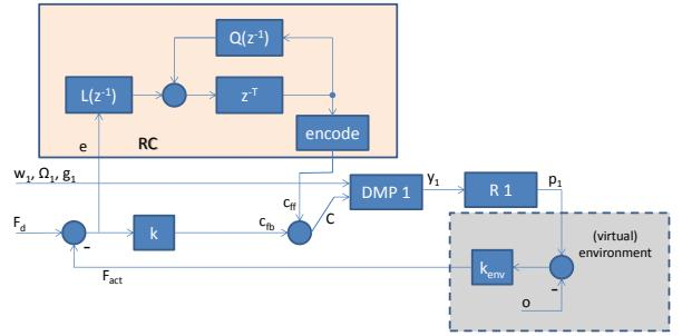
Fig. 1. Schematic of the RC in combination with the DMP and the robot (R1). Contact with the environment provides the force  $F_{\text{act}}$ . The force can be the real, measured force, or a virtual force calculated with (9).
