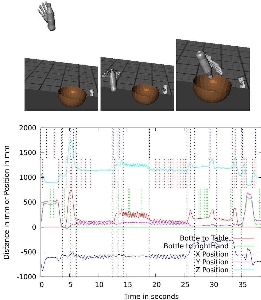
Figure 3.6: Right: Comparison of manual segmentation (black lines), the proposed approach (blue lines, PCA (red lines) and Zero-Velocity-Crossing (green lines) of an action sequence shown by the key frames (vertical lines). The action sequence contains grasping, placing, shaking, tossing, pouring, inspecting and dripping off a bottle. The vertical lines are only partly drawn for better clarity. Left: Snapshots of the segmented action sequence for visualization.
