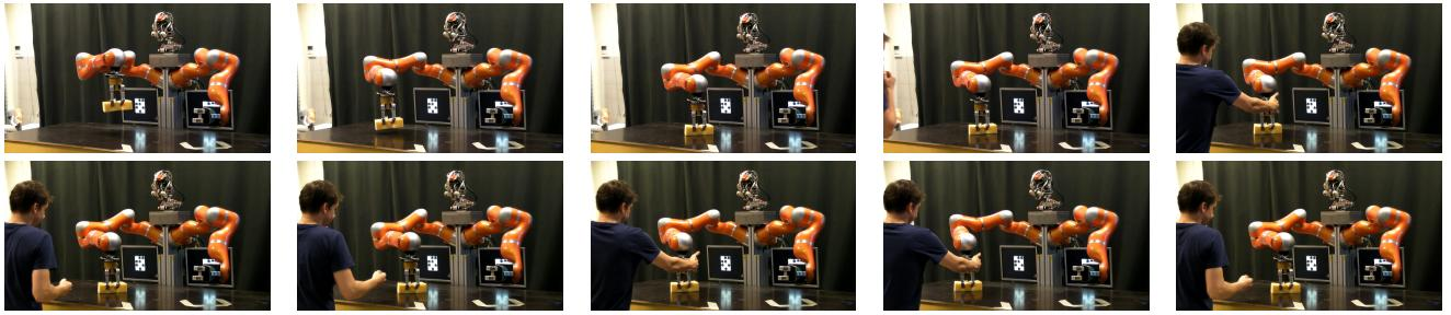
Fig. 8. Sequence of images showing on-line coaching of robotic motion using force feedback while the robot is maintaining contact with the table. The experiment is also presented in the video and its results in Figs. 6 and 7.
