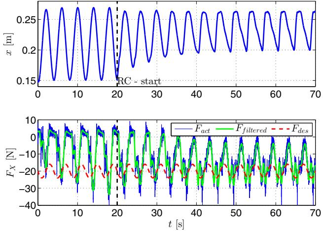
Fig. 6. Results of modifying the arm trajectories for a cooperative bimanual task of rotating the pedal racer with arms. The top plot gives the trajectory of the arm with  $x$  denoting the distance from the body to the tip of the arm. The bottom plot gives the estimate of the measured force (blue), filtered force (green) and desired force (red dashed).
