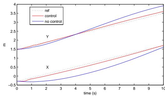
Figure 2.7: Results of the chair pushing along the straight line with and without the chair controller
