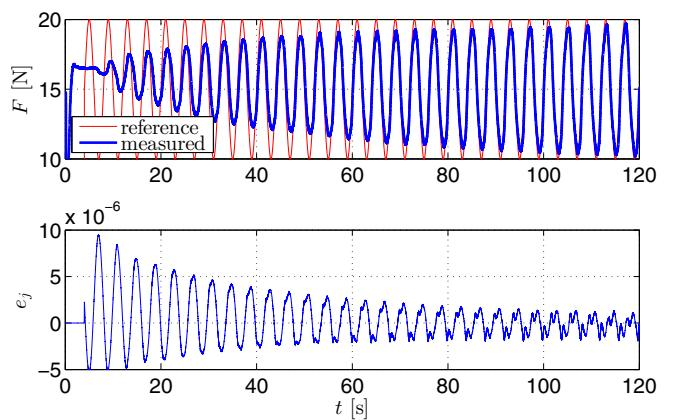
Fig. 5. The results of adapting the robot trajectory using 14, with a sinusoidal referential force. The experiment started with the robot already in contact with the surface. The referential and resulting forces are in the top plot, while the error signal, which is an input to the weight fitting, is in the bottom plot.
