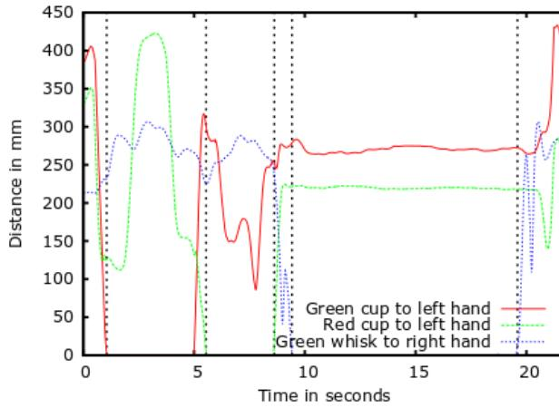
Fig. 6. Segmentation based on object contact relations: When two objects get in contact with each other (contact in this case is approximated as  $distance < 5mm$ ) or lose contact, a new key frame is inserted with the current world state attached to it. The dotted vertical lines depict the detected segments. Only distances between objects that get in contact during the complete demonstration are shown.
