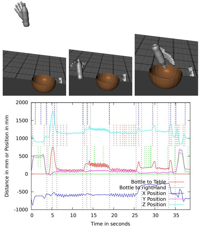
Fig. 8. Bottom: Comparison of manual segmentation (black lines), PCA (red lines), Zero-Velocity-Crossing (green lines) and the proposed approach (blue lines) of an action sequence shown by the key frames (vertical lines). The action sequence contains grasping, placing, shaking, tossing, pouring, inspecting and dripping off of a bottle. Top: Snapshots of the action sequence for visualization. The vertical lines are only partly drawn for better clarity.
