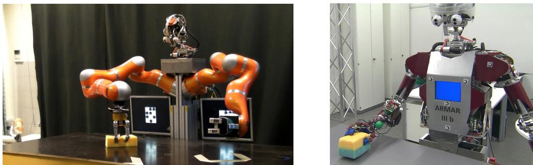
Figure 2.1: Table wiping using the KUKA robotic platform at JSI on the left and using the ARMAR humanoid robot on the right.
