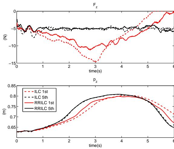
Fig. 4. Comparison of the real world experiments performed with ILC and RRILC. Upper graph shows the force tracking in  $Z$  direction. Lower graph shows the learned  $Z$  coordinate of the surface.
