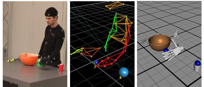
Fig. 5. All stages of the action sequence demonstration capture processing: (left) The human demonstrator with attached markers on the objects; (middle) marker group representation; (right) 3D mesh models with applied 6D object pose.
