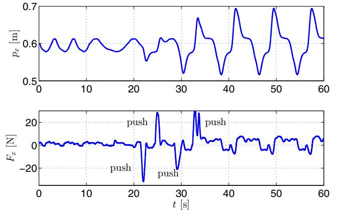
Fig. 7. The top plot depicts the trajectory of motion in  $x$  direction of the end effector of the robot. The external forces applied by the tutor, depicted in the bottom plot, modified the motion to achieve the intended result.
