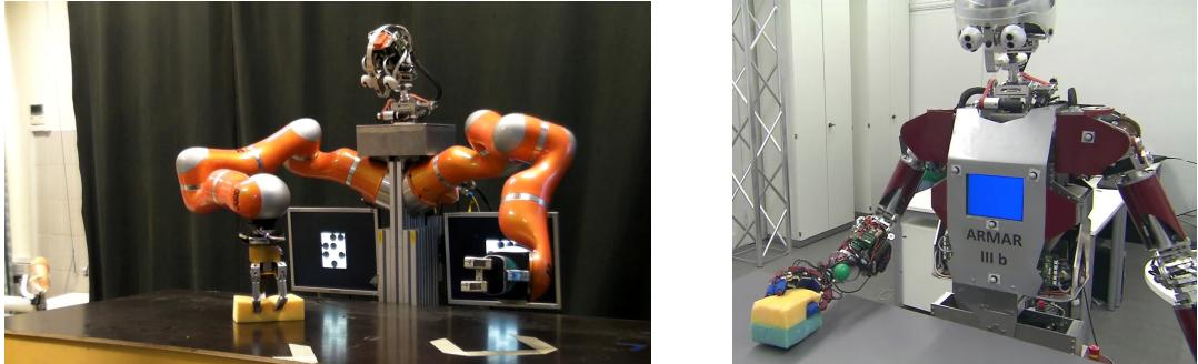
Figure 2.1: Table wiping using the KUKA robotic platform at JSI on the left and using the ARMAR humanoid robot on the right.
