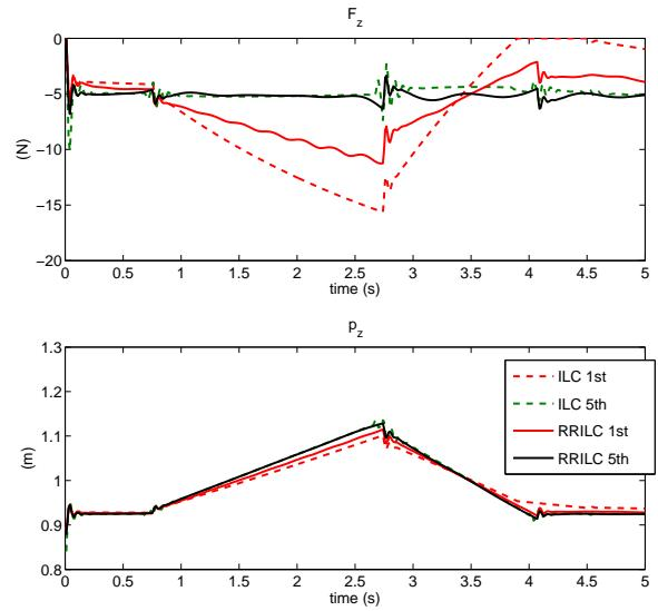
Fig. 2. Comparison of simulation results obtained with ILC and RRILC. Upper graph shows the force tracking in Z direction. Lower graph shows the learned Z coordinate of the surface
