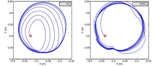
Fig. 6. Comparison of the learned trajectory for pot stirring obtained with RC (left) and RRRC (right).
