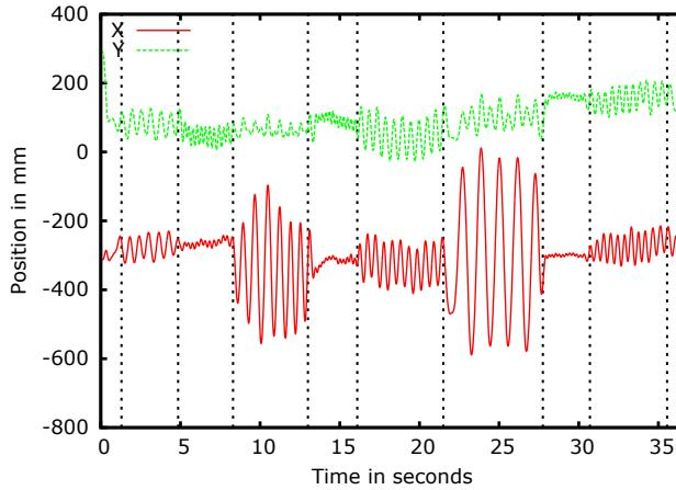
Fig. 7. Subsegmentation of one semantic segment (sponge touches hand and table) into different subsegments, i.e. different wiping styles. The z-dimension is omitted in the figure. The dotted vertical lines depict the segmentation points. Whenever the wiping styles changes, a key frame was inserted.
