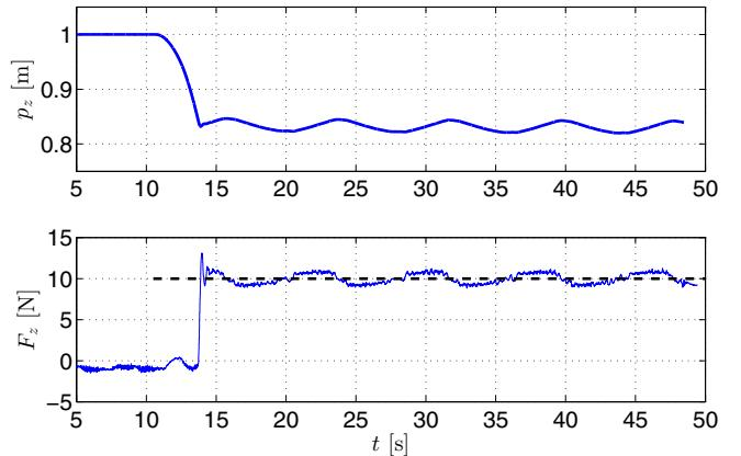
Fig. 3. The trajectory of motion when adapting to a flat but tilted surface in the top plot. The resulting forces show a clear hysteresis resulting from moving up or down the slope in the bottom plot. Fig. 2-right shows the complete 3-D trajectory arising in this experiment.
