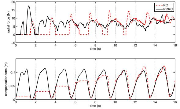
Fig. 5. Comparison of the experimental results for pot stirring obtained with RC and RRRC. Upper graph shows the force tracking in radial direction. Lower graph shows learned compensation term in radial direction. Dotted vertical lines denote stirring cycles.
