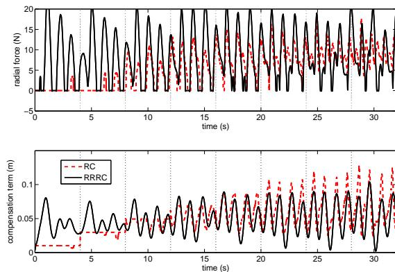
Fig. 8. Comparison of the experimental results for stirring in square pot obtained with RC and RRRC. Upper graph shows the force tracking in radial direction. Lower graph shows learned compensation term in radial direction. Dotted vertical lines denote stirring cycles.
