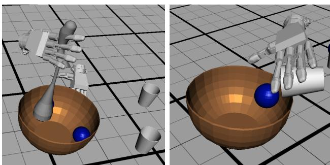
Fig. 4. Simulation of the observed demonstration while mixing with a whisk (left) and pouring from a cup (right).
