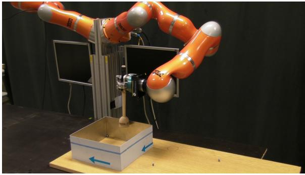
Fig. 7. Experimental setup for stirring in square pot.
