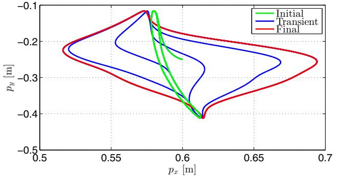
Fig. 6.  $X - Y$  plot of the end-effector motion depicts the initial motion in green, the motion during tutoring in blue and the final trajectory in red.
