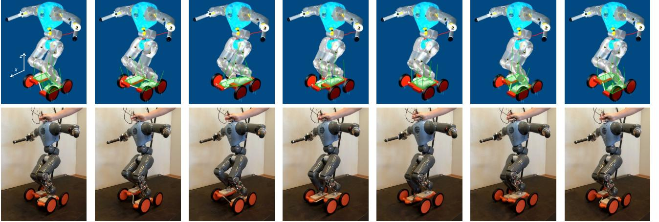
Fig. 8. In the top row an image sequence of one period of virtual COMAN steady-state pedaling on a virtual pedal racer in Webots dynamic simulator, after learning. The bottom row shows the real COMAN robot pedaling on the device. Note that the robot was helped to maintain balance at least once per period.
