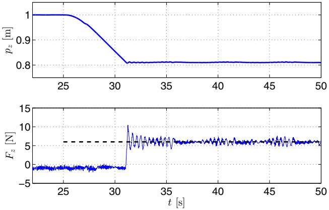
Fig. 1. The top plot shows real world results of adaptation of motion in  $p_z$  direction (downwards). The resulting forces with the referential force of contact given at 6 N (dashed line) is shown in the bottom plot. As the robot was performing left-right wiping motion, some oscillations due to the contact are visible in the force measurement. Fig. 2 left shows the complete 3-D trajectory for this experiment.
