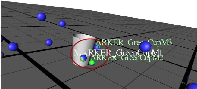
Fig. 3. Mapping of observed markers (blue spheres) attached to the cup to virtual markers on the model. Both, observed and virtual markers, are aligned (green/blue spheres in red circle). The visualization of the cup's 3D mesh shows the 6D pose of the perceived object.
