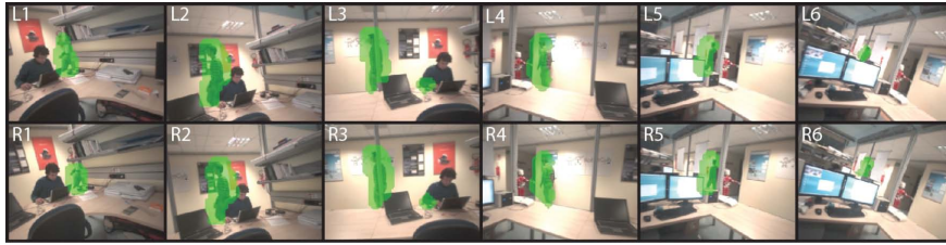
Figure 4.12: A sequence of images recorded during the real time stereo tracking of a person walking in front of the iCub: six images are shown in temporal order from L1 to L6 (left camera) and R1 to R6 (right camera). The walking person is highlighted with a green blob using the result of proposed algorithm.
