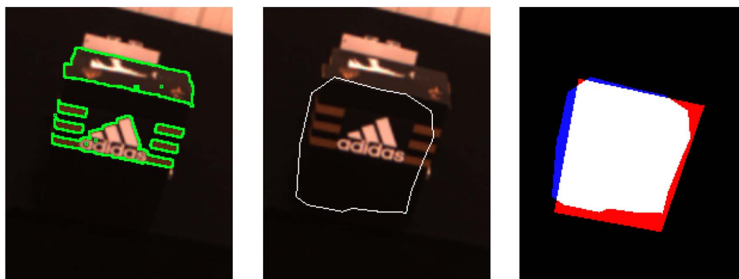
Figure 3.5: Results of the visuo-haptic exploration approach in figure-ground segmentation tasks. Due to ambiguities in the visual appearance of background and object the segmentation of the object based on visual data alone is affected (left). By enhancing the visual information using the proposed haptic exploration approach, the segmentation becomes more stable (middle). Compared to the ground truth, the visuo-haptic exploration approach is able to recover major parts of the contact surface (right).
