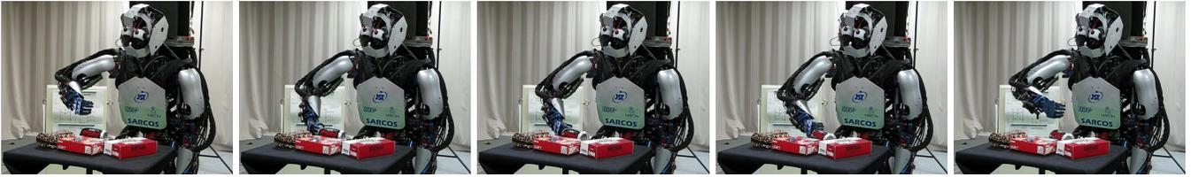
Fig. 5. A successful probing push. The robot starts at the position above the object, moves to the starting position for pushing, applies the probing pushing movement, and withdraws to the position above the object. All movements are generated using linear, autonomous dynamic systems. After the push the robot removes the arm from the viewfield to allow for unobstructed acquisition of the object image.
