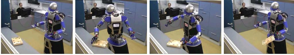
Figure 11: Execution of the plan involving the OACs **PlanPush**, **AgnoPush**, **PlanGrasp**, and **ObjGrasp**. From left to right: (1) the object is not graspable, (2) pushing moves the object into a graspable pose, (3) the object is grasped, and (4) the object can finally be picked up by the agent.
