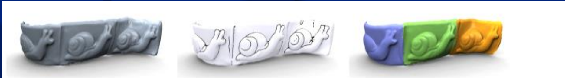
Figure 1.1: A 3D scan of a deformed plasticine sculpture with three snail figures. Our algorithm detects symmetries by looking at constellations of surface feature lines. This can be used for detecting deformable symmetries. Left: input data, middle: feature lines overlay, right: detected symmetries.
